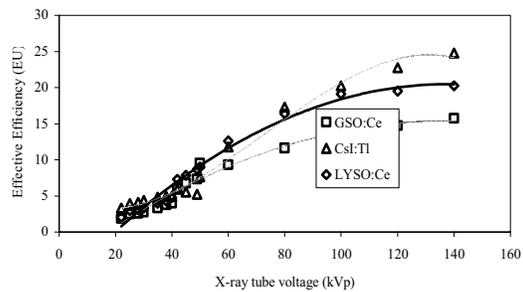
Figure 6. Effective efficiency of LYSO: Ce, GSO: Ce and CsI: Tl crystals using Si/S1133 crystalline silicon Hamamatsu photodiode.
