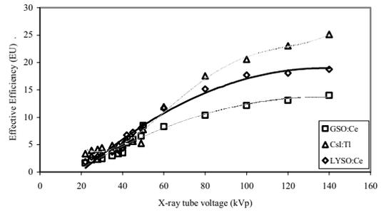
Figure 5. Effective efficiency of LYSO: Ce, GSO: Ce and CsI: Tl crystals using aSi:H-108H amorphous silicon photodiode with intrinsic layer thickness 800nm
