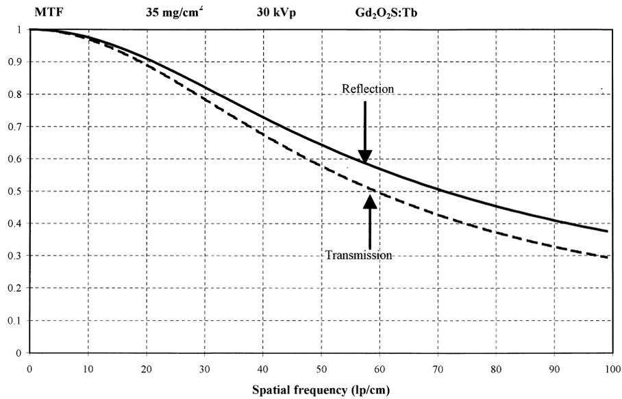
Fig. 3. Modulation transfer function of the 35 mg/cm<sup>2</sup> Gd<sub>2</sub>O<sub>2</sub>S:Tb scintillator layer in reflection and transmission mode.
