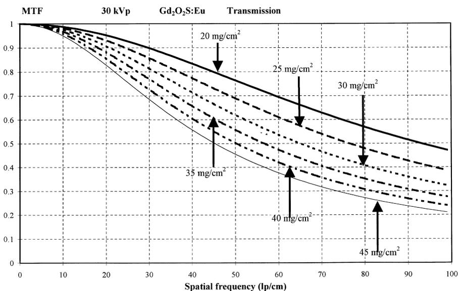
Fig. 2. Modulation transfer function of Gd<sub>2</sub>O<sub>2</sub>S:Eu scintillator for various coating weights, determined in transmission mode.
