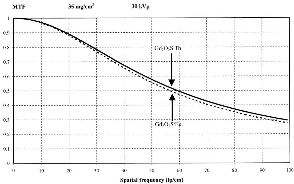
Fig. 4. Comparison of the modulation transfer functions of Gd<sub>2</sub>O<sub>2</sub>S:Tb and Gd<sub>2</sub>O<sub>2</sub>S:Eu scintillators determined in transmission mode.
