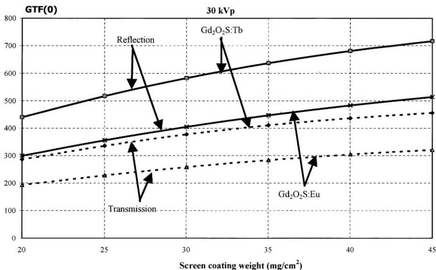
Fig. 1. Variation of the zero-frequency gain transfer function (emitted light photons/incident X-ray photon) of  $Gd_2O_2S:Tb$  and  $Gd_2O_2S:Eu$  scintillators, with increasing coating weight, determined in transmission and reflection mode at 30 kVp (approximately 18 keV average X-ray energy).
