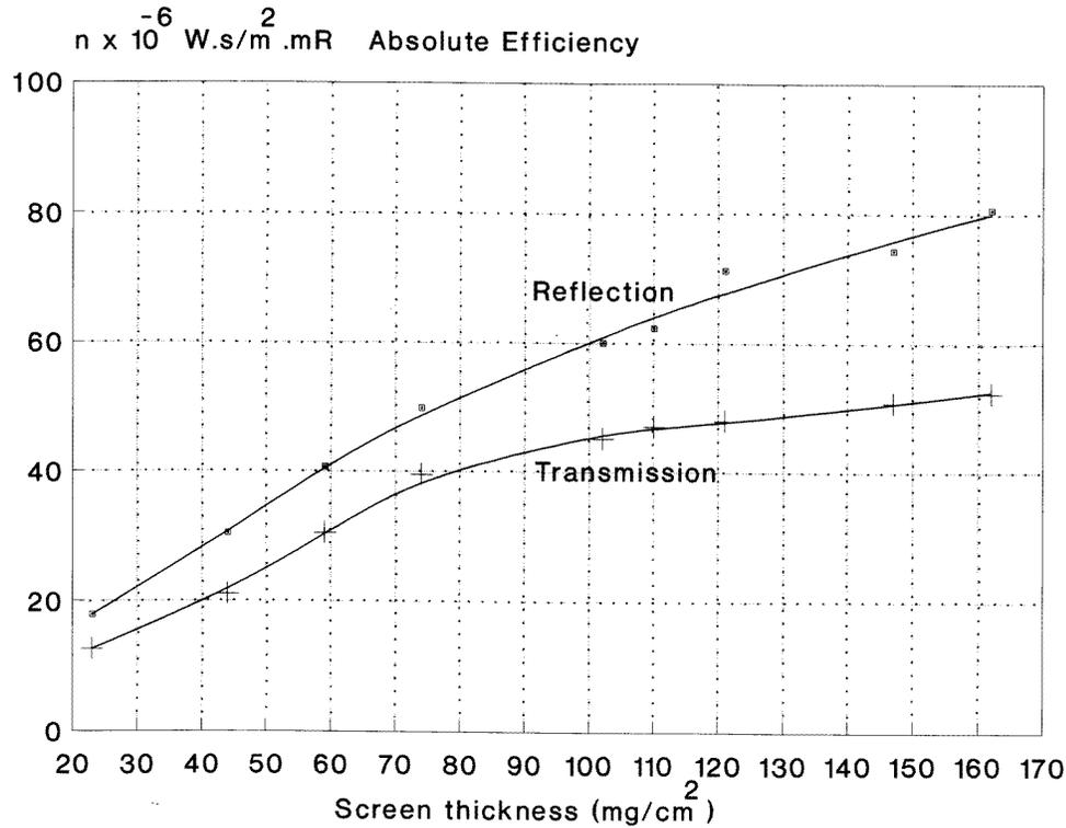
**Figure 4.** Absolute efficiency of La<sub>2</sub>O<sub>2</sub>S:Tb screens versus screen's coating thickness for both reflection and transmission mode, for 80 kVp x-ray tube voltage. Solid lines, theoretical results; points, experimental data.
