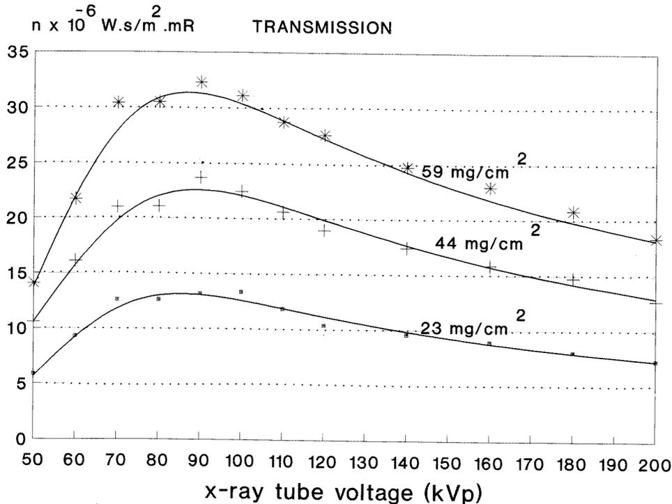
**Figure 2.** Absolute efficiency in transmission mode versus x-ray tube voltage for three La<sub>2</sub>O<sub>2</sub>S:Tb screens of 23, 44, and 59 mg cm<sup>-2</sup> coating thickness. Solid lines, theoretical results; points, experimental data.
