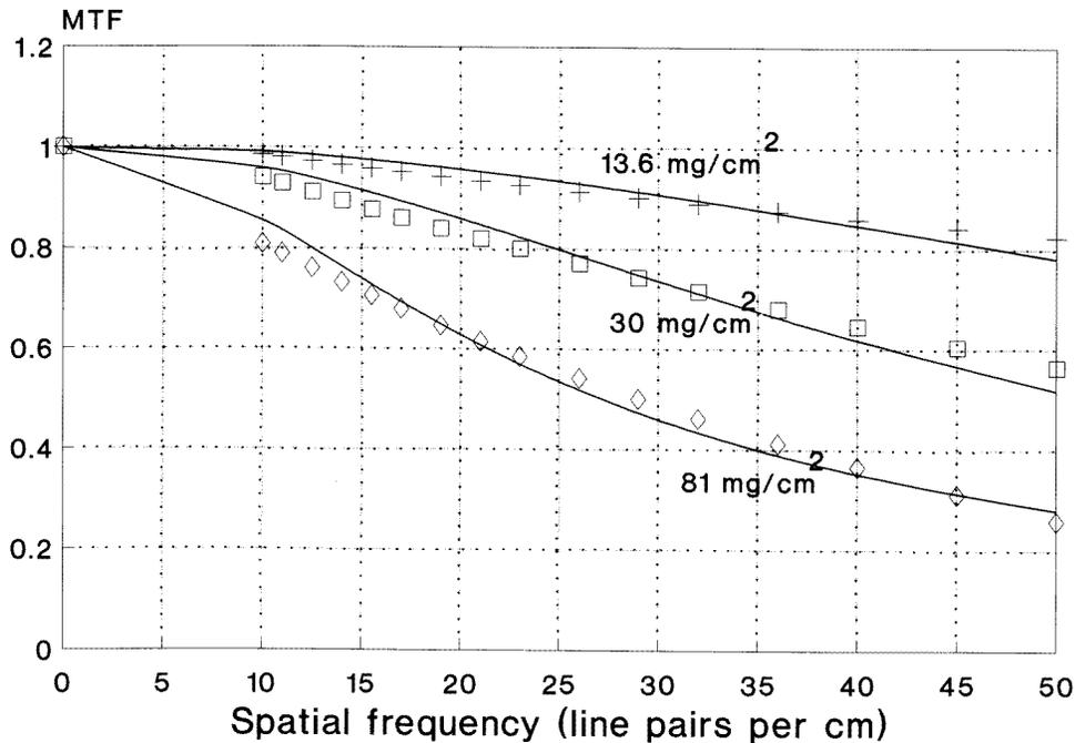
**Figure 6.** MTF curves for three La<sub>2</sub>O<sub>2</sub>S:Tb screens of 13.6, 30, and 81 mg cm<sup>-2</sup> coating thickness. Solid lines, calculated MTF values; points, experimental data.
