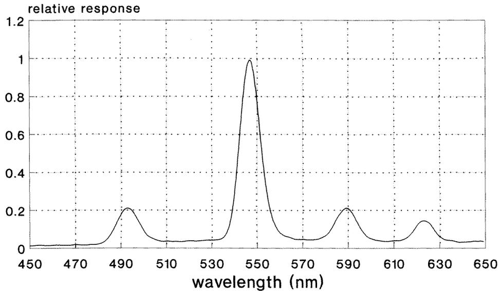
Figure 1. The spectral response of the  $\text{La}_2\text{O}_2\text{S:Tb}$  screen.
