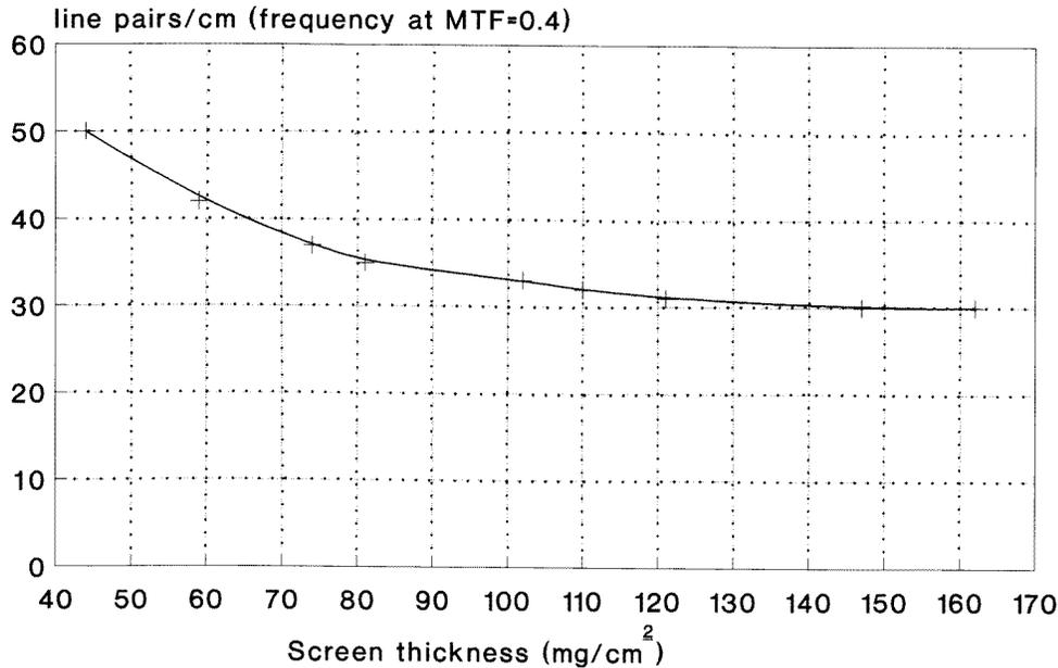
**Figure 8.** Calculated values of resolution (frequency at MTF = 0.4) against screen coating thickness for La<sub>2</sub>O<sub>2</sub>S:Tb screens.
